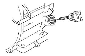
Figure 4. Engine Oil Dipstick (Removal)
